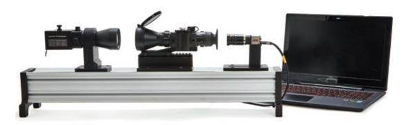
OE-710, Collimator is an optical system designated for Night Vision Sight testing. The OE-710, collimator enables performing resolution, reticule balanced and Clicker movement tests, with high accuracy results either for final assemble or as a maintenance routine.
