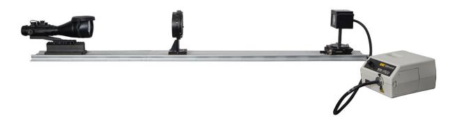
OE-700, Collimator is an optical system designated for Night Vision Sight (weapon sight and clip-on sight) testing and calibration. The OE-700, collimator enables performing resolution and field of view tests with high accuracy results either for final assembly or as a maintenance routine.
