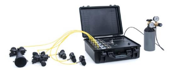
Nitrogen purging system is an electric kit that enables performing nitrogen purge, fill up and leak test for five Night Vision Devices simultaneously. Nitrogen purging and leak test is required for final assembly and as a basic Night Vision Devices maintenance measure in order to keep the interior part dry and clean. With Tesoptics' nitrogen purging and leak system this operation is fast, simple and safe.
